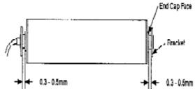
The Motorized Pulley supports bracket grooves must be well aligned and both parallel, allowing for a max gap of the shaft/end-caps slots of max 0.2 mm.
